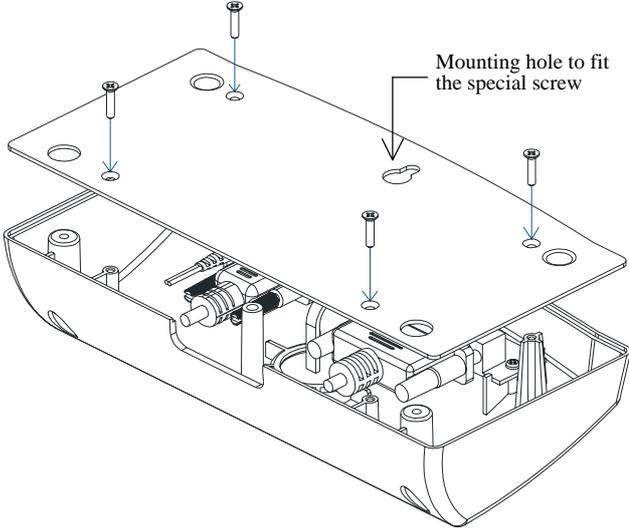
6. You may use the enclosed mounting screws (one Special screw and two Wood screws) to fix the Display on the wooden table surface.
