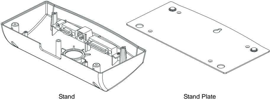
2. Get the DISPLAY unit and place the Cable from the Display through the extension pillars to the Stand.
