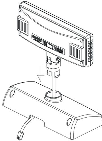
4. Connect the cable from the Display to the RJ connector (TO DSP) inside the Stand until you feel it clicked.
